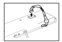
Remove the CCD Assy Cover. (loosen the four screws)
